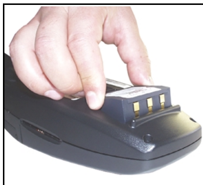
Figure 2-3. Installing the ICE 4000 Battery Pack
