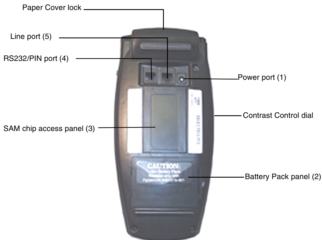
Figure 2-8. ICE 4000 under panel connectors
