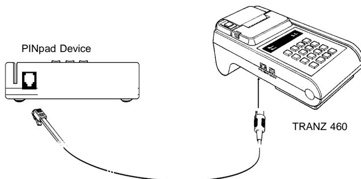
Figure C-2. PINpad Device to TRANZ 460 Connection
