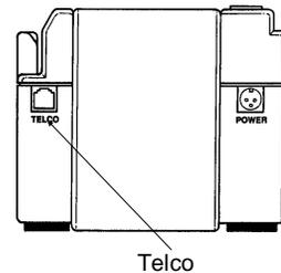
Figure 3-9. Telephone Connection
